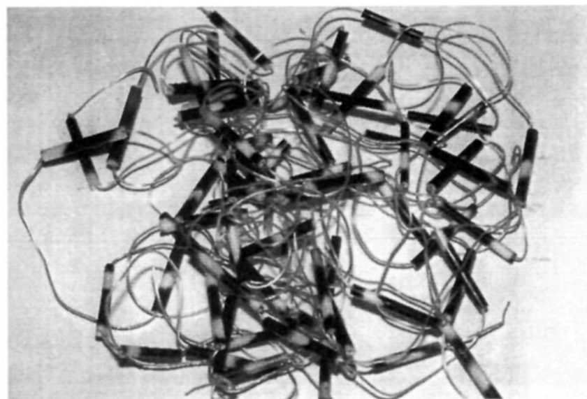
Figure 6. Model of the supramolecular structure and morphology of the rod-coil copolymers at one composition f .
